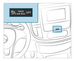
Vehicles without automatic co-driver airbag shutoff have a special sticker affixed to the side of the cockpit on the co-driver side ( $\rightarrow$  page 42).
