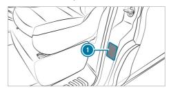
Vehicle identification plate (1) is on the B-pillar on the driver's side.
