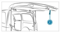
To close: pull the tailgate firmly downwards by loop ② and close it from outside.
