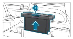
To fold out the table panel: pull out the table panels upwards to the stop using handles @ and swing them to the side until they engage.
