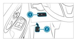
If, in exceptional cases, the service brake fails, you can use the parking brake to perform emergency braking.
