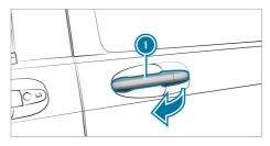
The sliding door is equipped with an active retainer, which engages when the door is opened as far as it will go.
