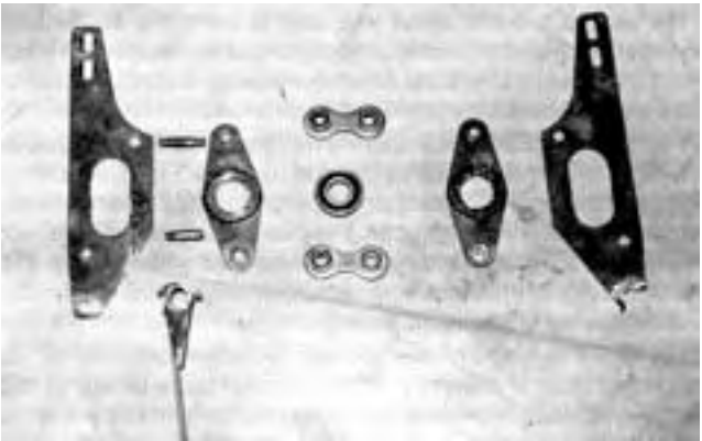
FIGURE 4. Failed Knife Drive Mechanism.
