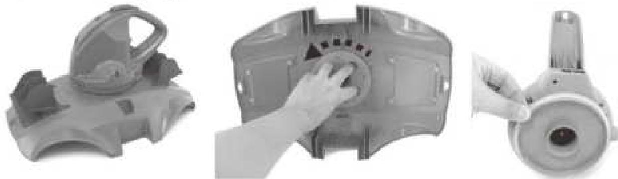
2. Use the screwdriver to unscrew the 4 screws located on the bottom of the head to release the bottom plate at first. Use the screwdriver to unscrew all the screws on the base as shown. Remove the impeller and then pry up the base and remove it to expose head inside.
