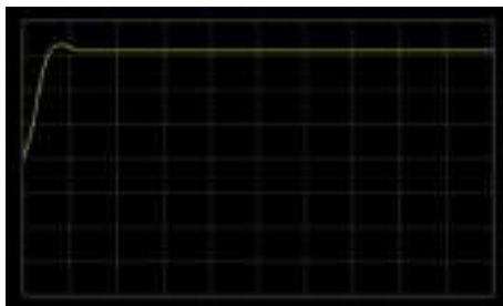
ARB 12 Second order impulse response(damping coefficient 0.1)
