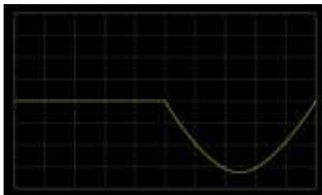
ARB 6 Sine wave, half-wave rectification(negative polarity)
