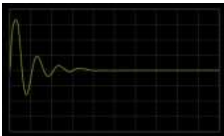
ARB 14 Second order impulse response(damping coefficient 0.7)
