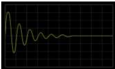
ARB 12 Second order impulse response(damping coefficient 0.1)
