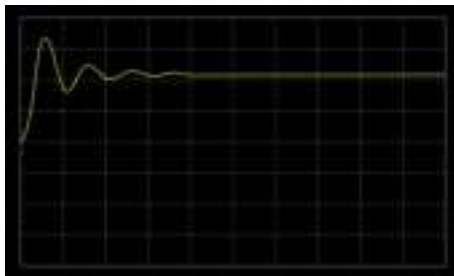
ARB 11 Second order step response(damping coefficient 0.7)
