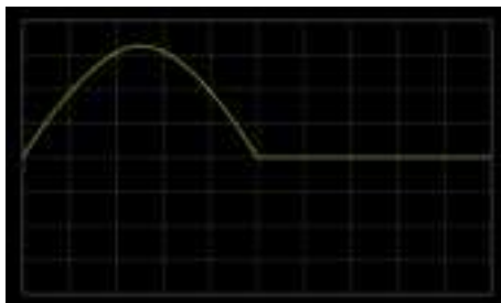
ARB 6 Sine wave, half-wave rectification(negative polarity)
