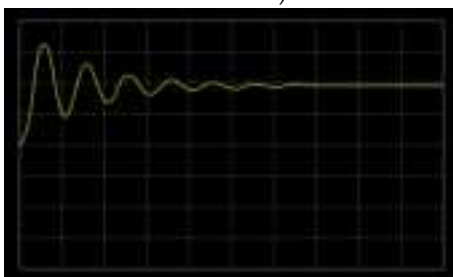
ARB 9 Second order step response(damping coefficient 0.1)
