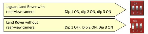
**Note:** On Land Rover setting dip 1 to ON codes the factory rear-view camera input which is located on the brown Fakra male connector of the factory monitor. When reverse gear is engaged, the navigation will automatically switch to this input. On vehicles with factory rear-view camera set Dip 1 to ON, too.
