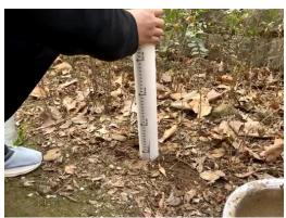
Notice: Installation should be done slowly, do not pull the sensor upwards to avoid air entering the hole and affecting the measurement.
