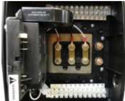
Figure 2: CoreSense Diagnostics sensor module located in terminal box
