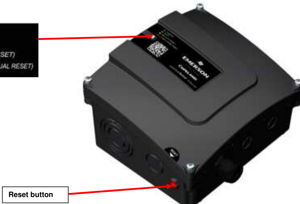
Figure 12: Copeland compressor electronics module terminal box with LED indicators and reset button
