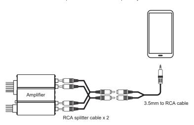
RCA connections are for input only and cannot be used as outputs.
