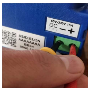
Figure 1 Checking DC voltage
