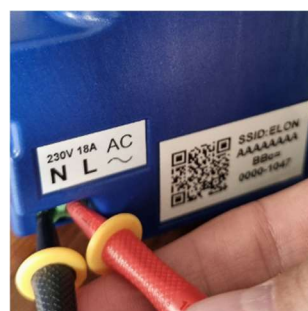
Figure 2 Checking AC voltage
