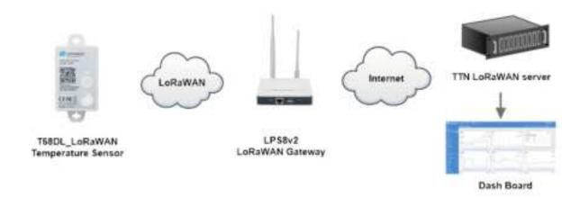
Assume the LPS8v2 is already set to connect to <u>TTN V3 network</u>, So it provides network coverage for T68DL. Next we need to add the T68DL device in TTN V3:
