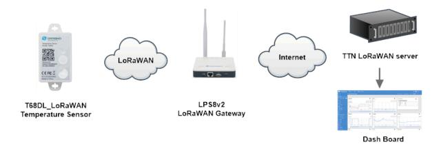
Assume the LPS8v2 is already set to connect to <u>TTN V3 network</u>, So it provides network coverage for T68DL. Next we need to add the T68DL device in TTN V3:
