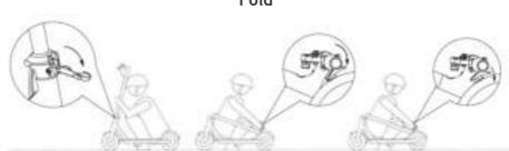
Make sure the scooter is turned off. Hold the front pole, lose a lock lever and lower a steering rack. Adding a steering rack in a horizontal position and secure it by inserting a hook through a special ring, which is located on the rear wheel mudguard. To Assemble the scooter, disconnect a steering rack lock from a hook of a mudguard, and then lift it into a vertical position and lock a lever.
