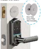
B. Remove the handle, lower the deadbolt, and install the lock above it.
