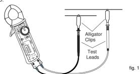
9. After measurement, turn off the power of the measuring circuit and discharge the all capacitors
