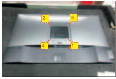
Wedge your fingers between the rear cover and the middle bezel on the corners of the top side of the monitor to release the rear cover, then use one hand to press the middle bezel, the other hand to pull up carefully the rear cover in order of arrow preference for unlocking mechanisms of rear cover.
