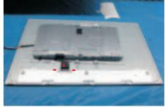
S14 Lift up the bracket chassis module and put it on a protector cushion.
