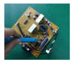
S17-4 Take out bulk cap. pin solder with soldering iron and absorber
