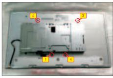
Release the panel cable by tearing off the adhesive tape, and then disconnect the panel power cable away from the connector of the panel module.
