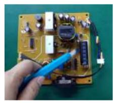
S17-3 Cut into the bottom of bulk cap. and pull it up carefully
