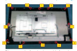
Disconnect the function key cable from the connector of the interface board, then tear off the adhesive tapes to release the function key cable.
