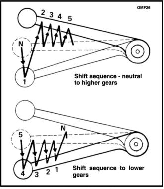
Figure 31. 5 - Speed Shifting Sequence
