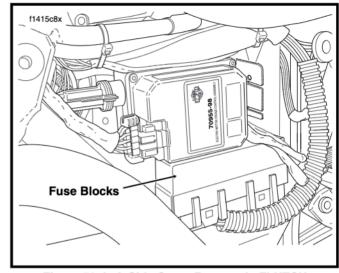
Figure 50. Left Side Cover Removed - FLHTCU
