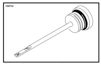
Figure 36. Transmission Lubricant Dipstick - 1340cc and 1450cc Models
