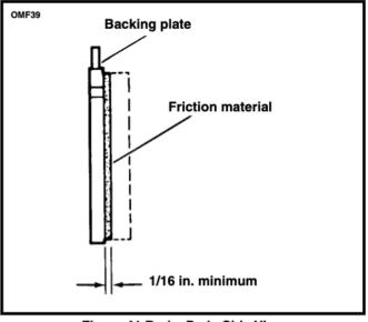
Figure 41.Brake Pad - Side View
