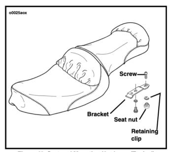
Figure 48. Seat and Mounting Hardware (Typical)
