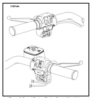
Figure 6. Sound System/Cruise Control Handlebar Controls
