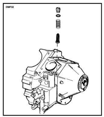
Figure 35. Hydraulic Lifter Oil Filter Screen
