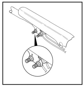
Figure 17. Air Suspension Adjustment Valves - FLT Models
