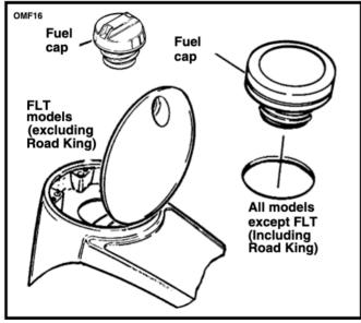
Figure 16. Fuel Filler Cap
