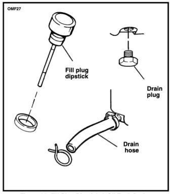
Figure 33. Fill Plug Dipstick & Oil Tank Drains
