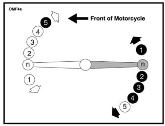
Figure 4. Gear Shifter
