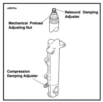
Figure 21. Front Suspension Adjustments
