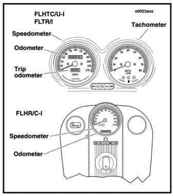
Figure 9. Speedometer, Odometer, Trip-odometer, Tachometer
