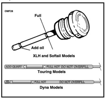
Figure 32. Engine Oil Level
