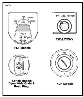
Figure 1. Ignition/Light Key Switch
