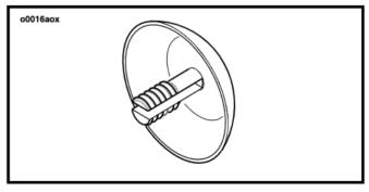
Figure 29. Seat mounting hole plug
