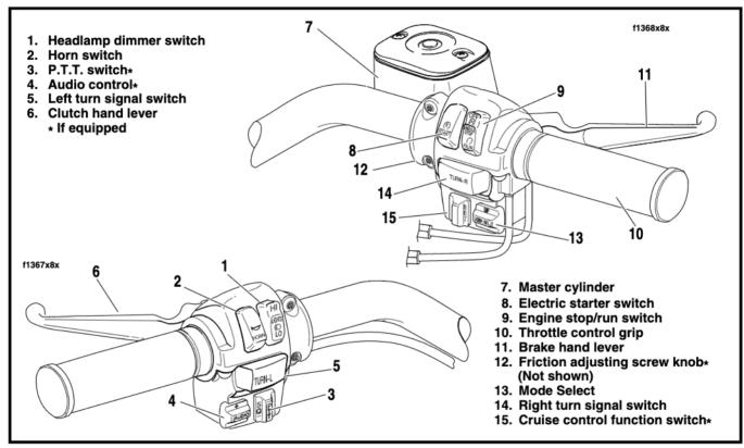
Figure 2. Handlebar Controls
