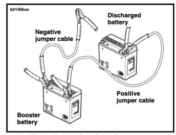
Figure 47. Jump Start Cable Connections
