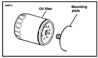
Figure 34. Engine Oil Filter
