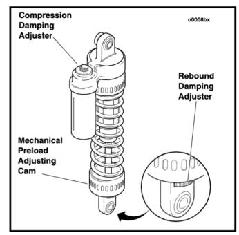
Figure 22. Rear Suspension Adjustments
