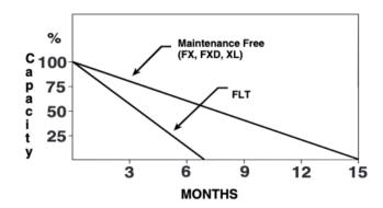
To reduce battery self discharge, remove and store the battery in a cool, (not freezing) dry place when the motorcycle is being stored.
