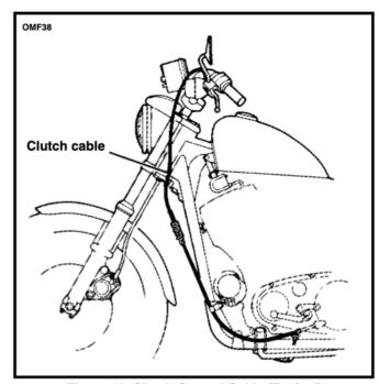
Figure 40. Clutch Control Cable (Typical)
