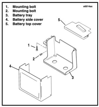
Figure 49. Dyna Glide Battery Tray and Mounting Hardware
