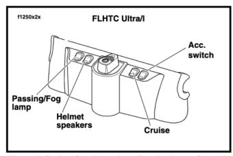
Figure 5. Cruise, Speakers, Acc., Passing Lamp Controls
