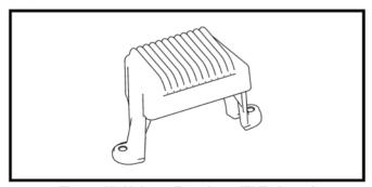
Figure 45. Voltage Regulator (FLT shown)
