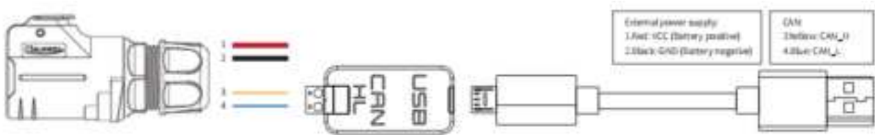
Figure 3.4 CAN connection diagram
