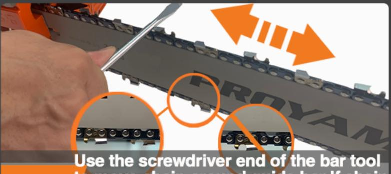
Use the screwdriver end of the bar tool to move chain around guide bar.If chain does not rotate, it is too tight. Slightly loosen bar nuts and loosen chain by turning the adjustment screw 1/4 turn counterclockwise.Retighten bar nuts.
