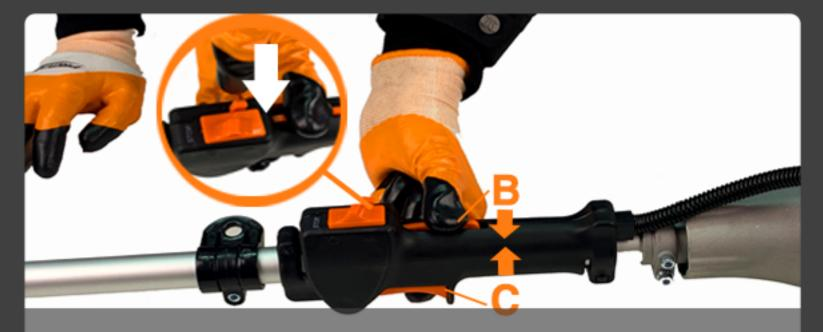
Push the throttle control lever B and the throttle safety lever at the same time C and keep them in this position whilst pressing the throttle shutter button
