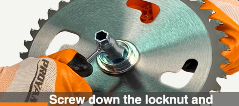
tighten it by turning the allen key counter clockwise.Remove Allen key and check for freedom of motion of the blade.
