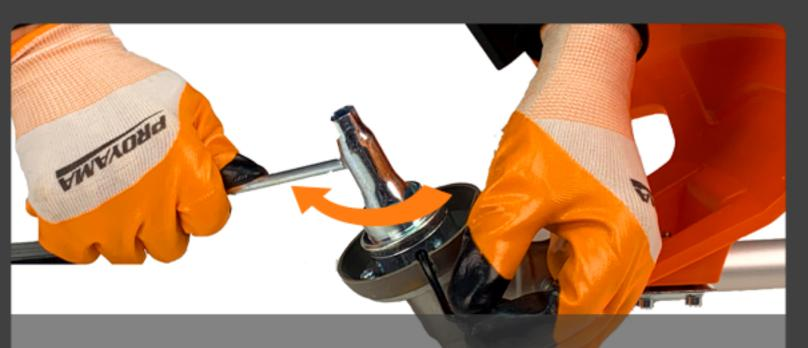
Unscrew the locknut (3) from the shaft by turning it clockwise with the spark plug wrench and screwdriver.
