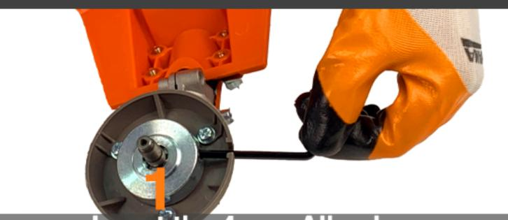
Insert the 4 mm Allen key through the winding guard and the mounting disc (1) into the opening on the angle gear (blocks the angle gear).
