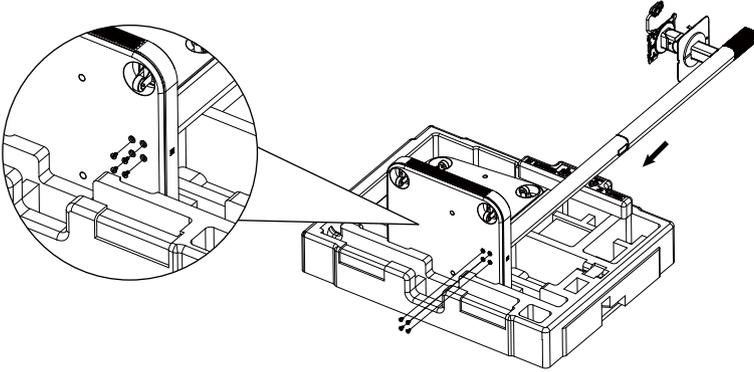
4. Hold the stand up, then assemble the display and stand. You could utilize the display "cavity slot" and stand "bracket hook" to hold the display easier. Put the power socket at "left side" position, then you can move the display to the stand bracket until you hear a click sound.
