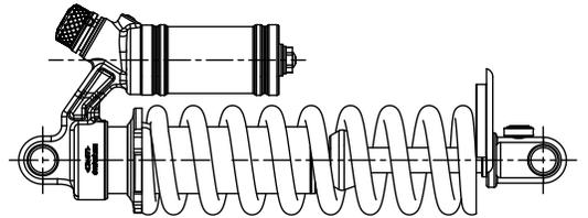
6. Tighten preload knob until safety ring and spring are tight
