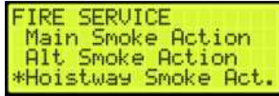
Figure 579: FIRE SERVICE Menu – Hoistway Smoke Action
