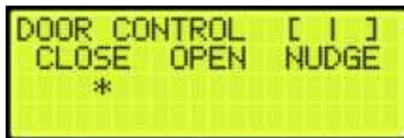
Figure 711: Enter Door Command Menu (Front Doors Only)
