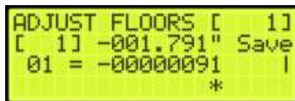
Figure 232: ADJUST FLOORS Menu – Too High
