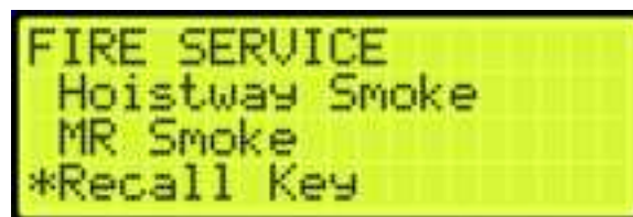
Figure 593: FIRE SERVICE Menu – Recall Key
