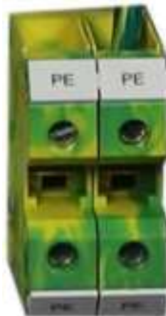
Figure 6: Ground Bus Terminal Blocks
