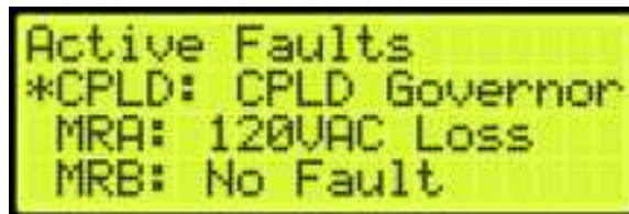
Figure 750: Active Faults Menu
