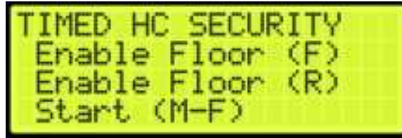
Figure 273: TIMED HALL CALL SECURITY Menu – Enable Floor (Front or Rear)
