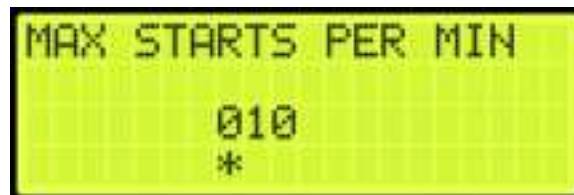
Figure 455: MAXIMUM STARTS PER MINUTE Menu
