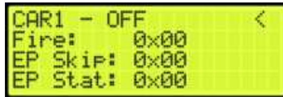
Figure 698: Fire Emergency Power Status Menu
