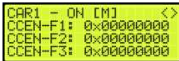
Figure 375: Front Car Call Enable Bitmap Status
