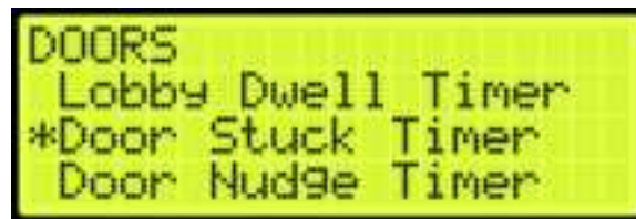
Figure 312: DOORS Menu – Door Stuck Timer
