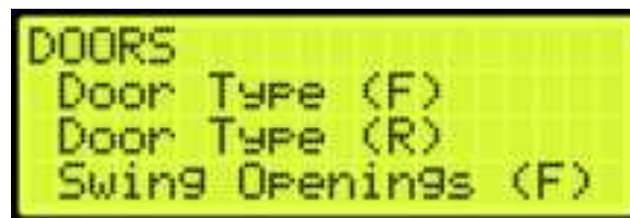
Figure 346: DOORS Menu – Door Type (Front or Rear)
