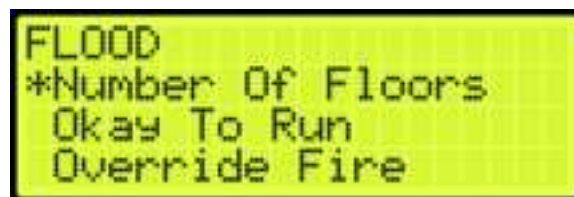
Figure 618: FLOOD Menu – Number of Floors
