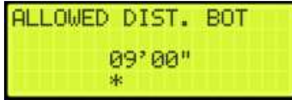
Figure 416: ALLOWED DISTANCE – BOTTOM Menu
