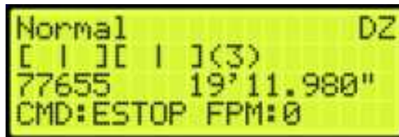
Figure 192: Check Status by Main Screen Method
