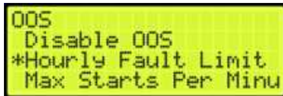
Figure 452: OOS Menu – Hourly Fault Limit
