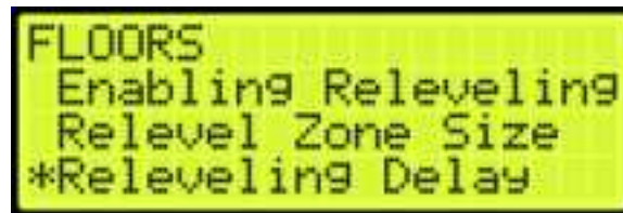
Figure 252: FLOORS Menu – Releveling Delay
