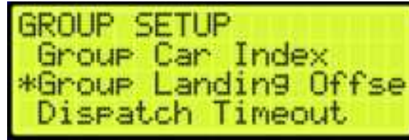
Figure 684: GROUP SETUP Menu – Group Landing Offset
