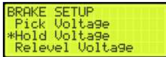
Figure 81: (Primary) BRAKE SETUP Menu – Hold Voltage
