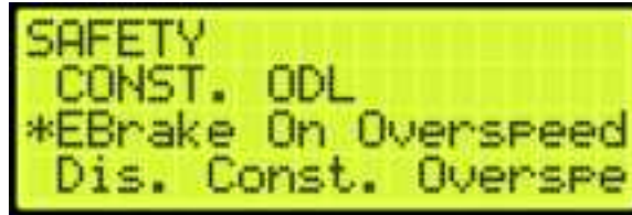
Figure 526: SAFETY Menu – EBrake On Overspeed
