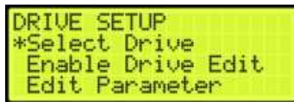
Figure 118: DRIVE SETUP Menu – Select Drive
