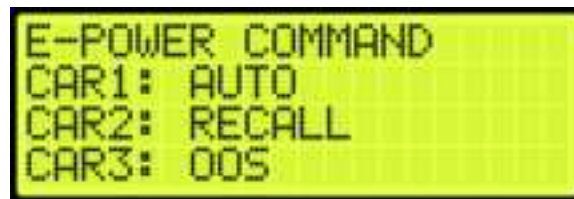
Figure 658: E-POWER COMMAND Menu
