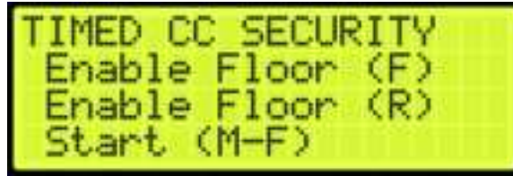
Figure 263: TIMED CC SECURITY Menu – Enable Floor (Front or Rear)
