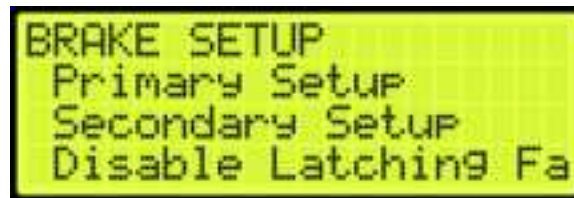
Figure 77: BRAKE SETUP Menu – Primary or Secondary Setup
