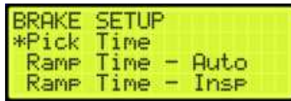
Figure 87: (Primary) BRAKE SETUP Menu – Pick Time
