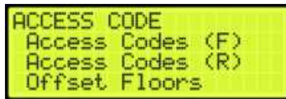
Figure 235: ACCESS CODE Menu – Access Codes (Front or Rear)
