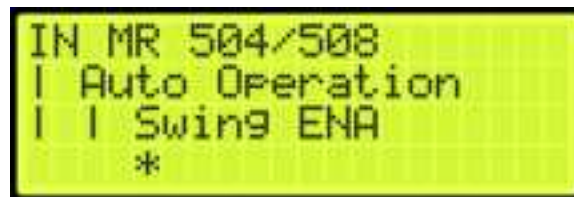
Figure 486: Input Menu – Enable Swing
