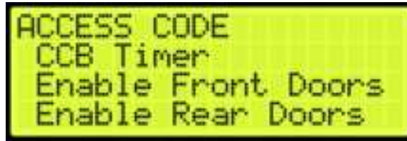
Figure 242: ACCESS CODE Menu – Enable Front (or Rear) Doors
