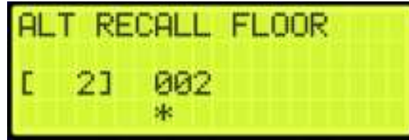
Figure 562: ALT RECALL FLOOR Menu
