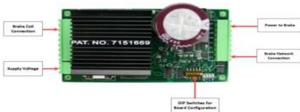
Figure 29: Brake Board SR3038
