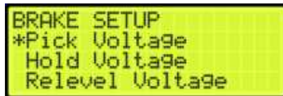
Figure 78: (Primary) BRAKE SETUP Menu – Pick Voltage
