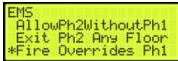
Figure 628: EMS Menu – Fire Overrides Ph1
