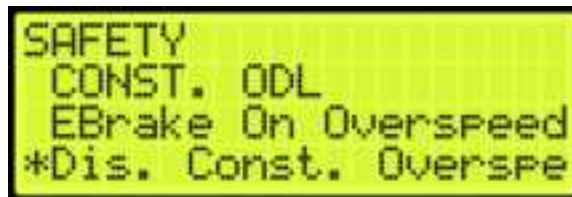
Figure 528: SAFETY Menu – Disable Construction Overspeed
