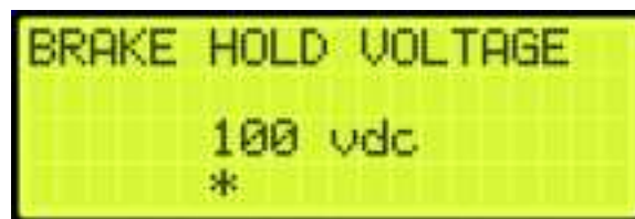
Figure 83: BRAKE HOLD VOLTAGE Menu
