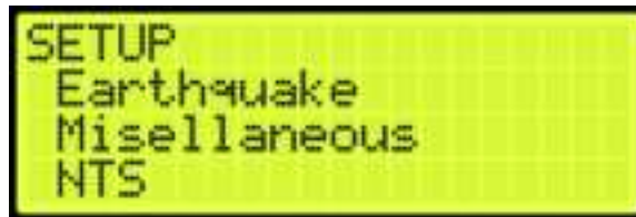
Figure 58: SETUP MENU – Earthquake, Miscellaneous, NTS
