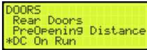
Figure 320: DOORS Menu – DC On Run
