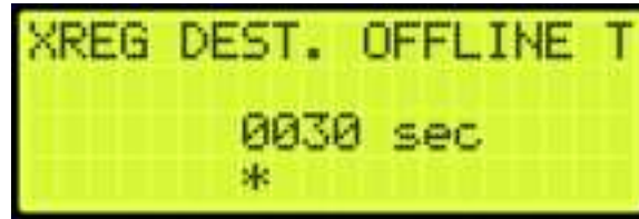
Figure 695: XREG DESTINATION OFFLINE TIMEOUT Menu
