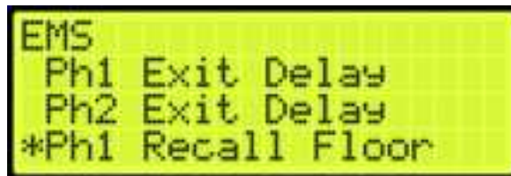
Figure 634: EMS Menu – Ph1 Recall Floor
