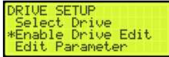
Figure 120: DRIVE SETUP Menu – Enable Drive Edit
