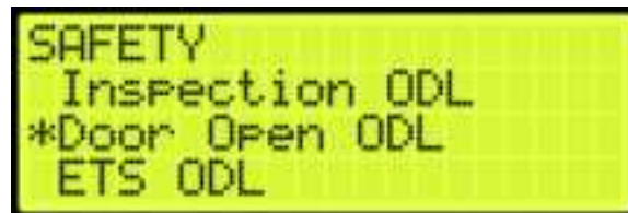
Figure 518: SAFETY Menu – Door Open ODL
