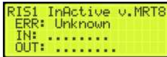
Figure 650: Inactive Riser Board Status
