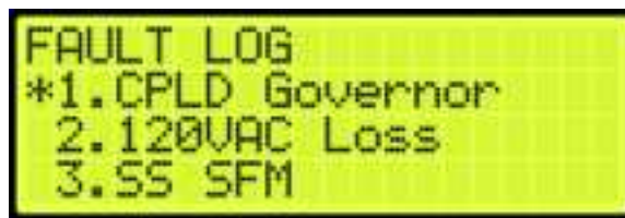
Figure 754: FAULT LOG Menu
