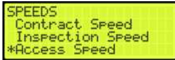
Figure 210: SPEEDS Menu – Access Speed
