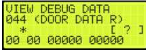
Figure 361: VIEW DEBUG DATA Menu – Rear Door
