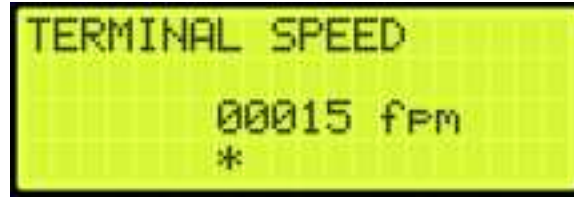
Figure 215: TERMINAL SPEED Menu
