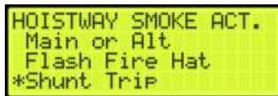
Figure 584: HOISTWAY SMOKE ACTION Menu – Shunt Trip
