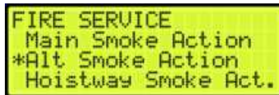
Figure 572: FIRE SERVICE Menu – Alt Smoke Action
