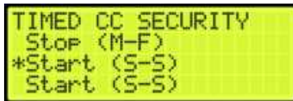
Figure 268: TIMED CAR CALL SECURITY Menu – Start (S-S)
