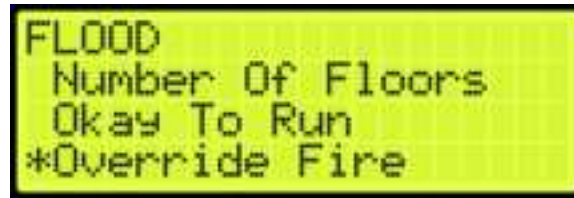
Figure 622: FLOOD Menu – Override Fire
