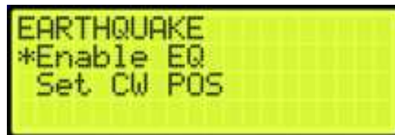
Figure 549: EARTHQUAKE Menu – Enable EQ
