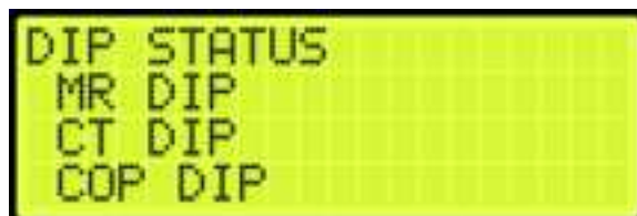
Figure 679: DIP STATUS Menu – MR, CT, or COP DIP
