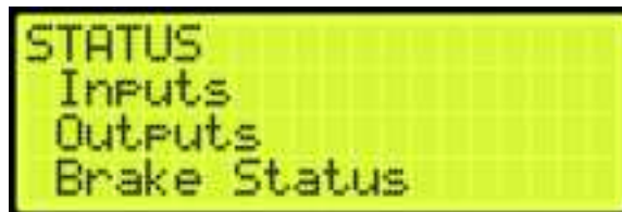
Figure 45: STATUS Menu – Inputs, Outputs, Brake Status
