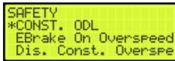
Figure 524: SAFETY Menu – Construction ODL
