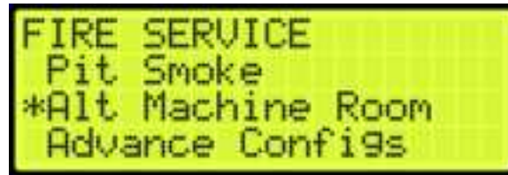
Figure 603: FIRE SERVICE Menu – Alt. Machine Room
