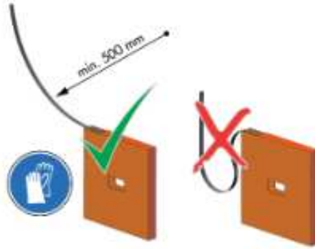
Figure 159: Tape Minimum Bend Radius
