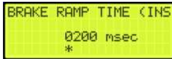
Figure 95: BRAKE RAMP TIME (INSPECTION) Menu
