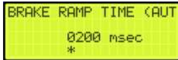
Figure 91: BRAKE RAMP TIME – (AUTO) Menu
