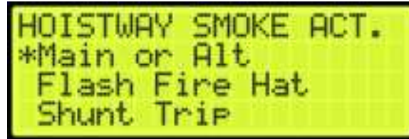
Figure 580: HOISTWAY SMOKE ACTION Menu – Main or Alt
