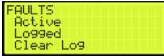
Figure 52: FAULTS Menu – Active, Logged, Clear Log
