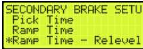
Figure 97: SECONDARY BRAKE SETUP Menu – Ramp Time – Relevel
