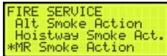
Figure 586: FIRE SERVICE Menu – MR Smoke Action
