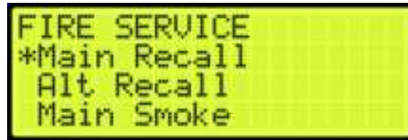
Figure 555: FIRE SERVICE Menu – Main Recall
