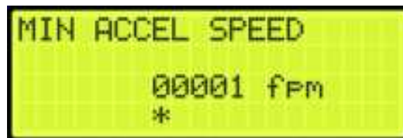
Figure 221: Minimum ACCEL SPEED Menu
