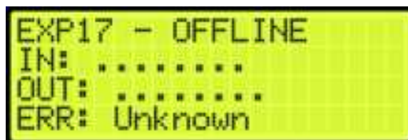
Figure 648: Inactive Expansion Board Status
