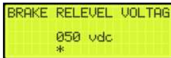
Figure 86: BRAKE RELEVEL VOLTAGE Menu
