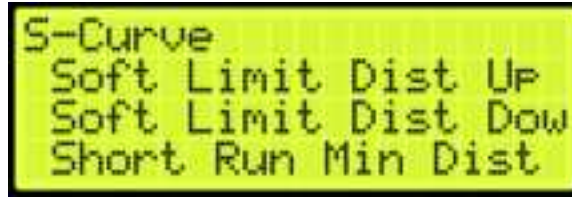
Figure 423: S-CURVE Menu – Soft Limit Distance (Up or Down)
