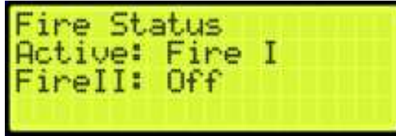
Figure 727: Fire Status Menu
