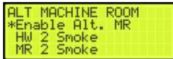
Figure 604: ALT MACHINE ROOM Menu – Enable Alt. MR
