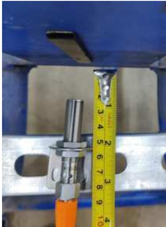
Figure 189: Mounting Proximity Sensor Assembly (Example)
