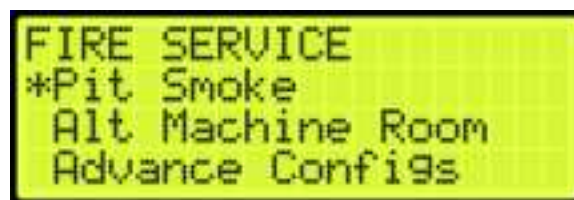
Figure 596: FIRE SERVICE Menu – PIT Smoke
