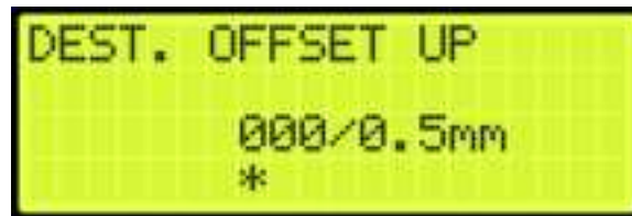
Figure 149: DESTINATION OFFSET UP Menu
