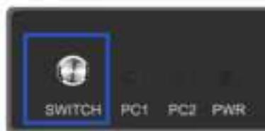
By toggle switching the front panel button, to switch PC1 and PC2.
