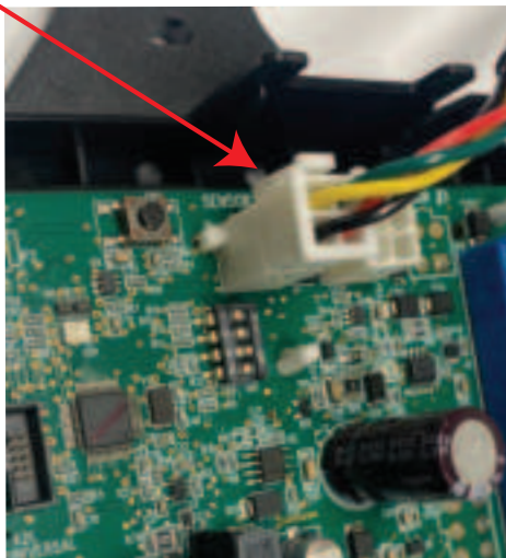
Figure 4. Connecting the RDS Sensor to RDS Blower Control Board
