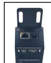
Network and Serial Connections located at the top of the unit.
