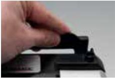
1. Open the cutter bar. For this, push the black handles at both sides of the cutter bar to the rear of the appliance.
