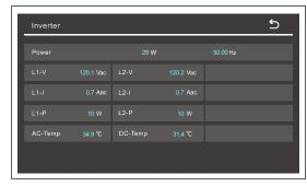
Inveretr Generation Power and Frequency. Voltage, Current, Power for each phase.
