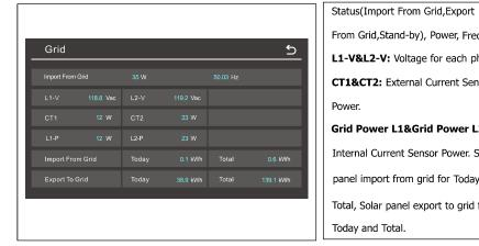
From Grid, Stand-by), Power, Frequency. **L1-V&L2-V:** Voltage for each phase. CT1&CT2: External Current Sensor Power. Grid Power L1&Grid Power L2: Internal Current Sensor Power, Solar panel import from grid for Today and Total, Solar panel export to grid for
