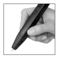
**3.** Put the filament in through the filament loading hole. Keep pressing or double click the filament loading button to load the filament.
