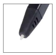
**6.** The pen will enter standby mode after 2 minutes of no operation. Click the filament loading button to start heating the pen. Please do not touch the tip of the pen.
