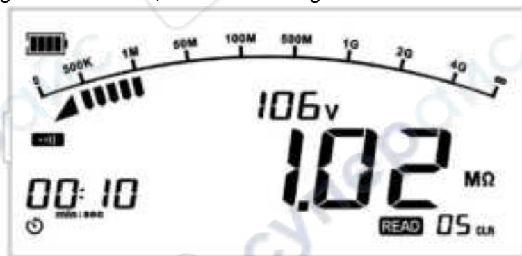
Figure 13.24 To delete the data of group 05 or all data
