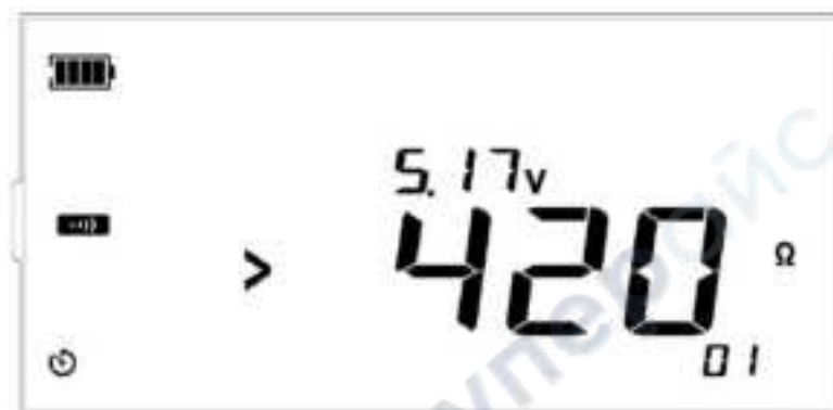
Figure 13.19 Low resistance exceeds the range
