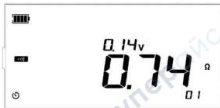
Figure 13.16 Test leads are shorted
