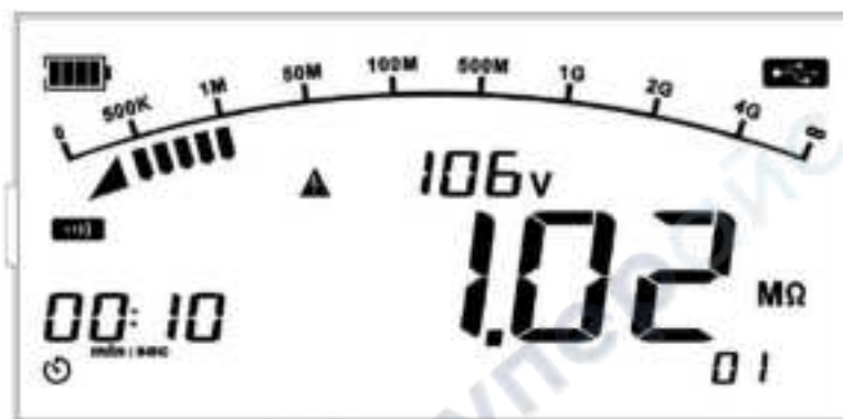
Figure 13.26 Real-time USB transmission in insulation measurement mode
