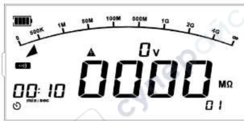
Figure 11.4 Test lead shorted
