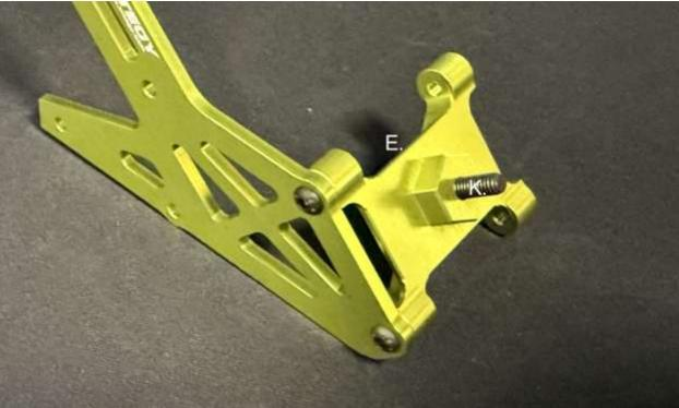
**STEP 6:** You should have an almost completed assembly. Finally, attach the remaining UPPER mount (C), LOWER mount (D), and LEFT-SIDE plate (A) to complete assembly.
