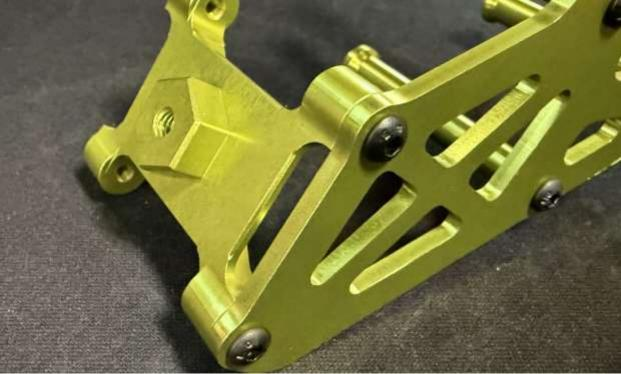
STEP 5: Thread 1x M4x20mm counter sunk screw (K) into the Spare Tire Mount (E); note that the counter sunk side of the mount matches the counter sunk screw head.
