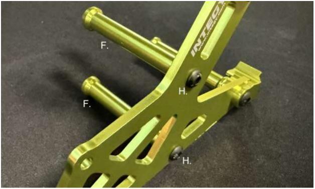
STEP 4: Attach Spare Tire Mount (E) to the RIGHT-SIDE plate using 2x M3x8mm button head screws (H) as shown. \*Pay attention to the hex hub direction of part (E).
