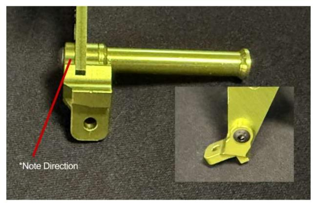
STEP 2: Attach 1x UPPER mount (C) to the RIGHT-SIDE plate (B) using 1x M3x12mm button head screw (I). Thread the screw into 1x 36mm post (G). \*Pay attention to the orientation of part (C).
