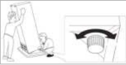
Slight unevenness in the floor can be leveled out using the front feet.
