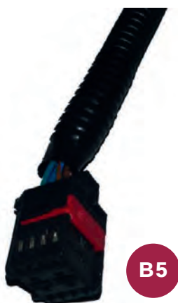
Figure 6 - Termination of the connection harness
