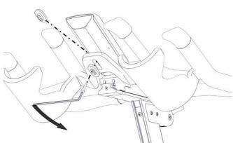
2. Remove the bolt from the BYOD bracket with a 2.5mm Allen key. The bolt will be used to fix the bracket to the handlebar at a later point.
