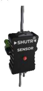
The **SHUTR Sensor** is simply clamped on to the power cord of a processing machine. It senses if the machine is powered on or off and will send a signal to the SHUTR network accordingly.
