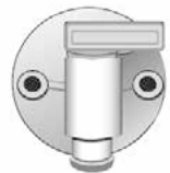
Exterior Fresh Water Drain
