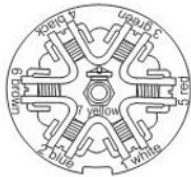
7-way trailer plug car end, rear view
