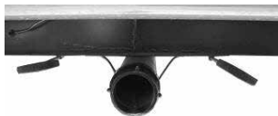
Black/Grey Tank Drain and Valves
