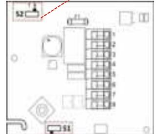
RFK 133/4 (Mat.-Nr. 1135006690) or RFW 103 (Mat.-Nr. 1135006689) (please order separately), then the slide switch must be moved to the right. The external sensor must be connected to terminals 7 and 8 (as shown in the connection diagram).
