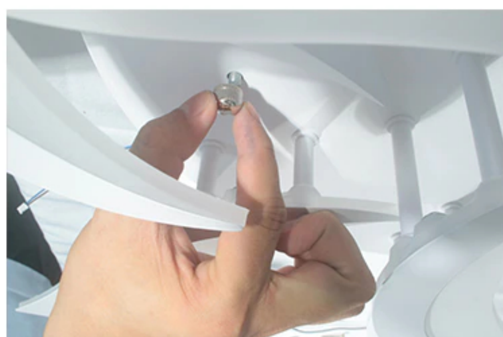
15:Lift up the light and install it to the cross, the four flat headed screws go through the plate and then use the nuts to fasten the light.
