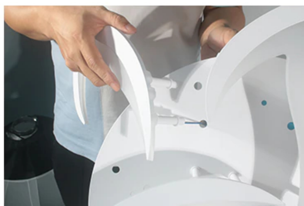
8: Assemble the petal with short tubes to the corner of the plate.
