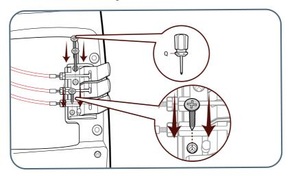
Place the seat mechanism (Part H) on the underside of the seat (ensure it is placed the right way round). Then tighten the seat mechanism using the mechanism screws provided (Part K) and the Allen key (Part 0).
