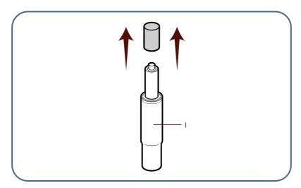
Then insert the gas spring (Part I) with the chrome rosette into the centre hole of the star base.
