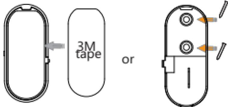
1. Use the double-side adhesive tape or the screws to fix the door sensor at the side of the door/window.
