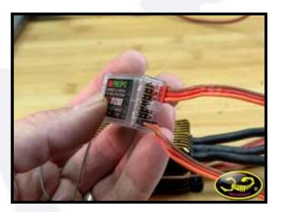
6.Remove propeller / pinion from the motor, check all connections, and apply suitable battery power to the ESC
