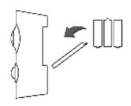
Open the battery door located at the back of Piper and insert the provided AA batteries. Close the battery door and secure it with the provided screw.
