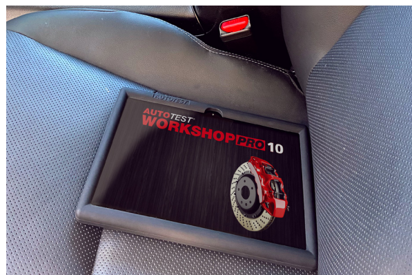
Figure 2: Workshop Pro in position ready for testing. If the unit is moving in the seat, place on the floor of the passenger seat. Supplied velcro will secure in place.
