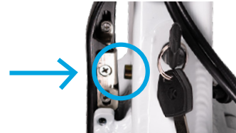
Locking Pin protruding through frame
