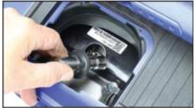
Figure 42 Remove the Spark Plug Boot
