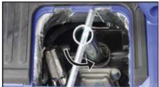
Figure 43 Remove the Spark Plug
