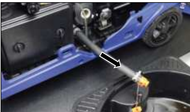
Figure 32 Draining the Engine Oil
