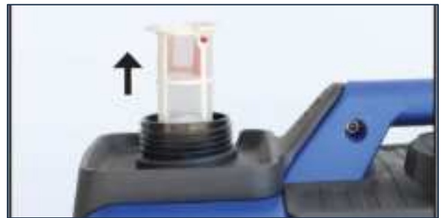
Figure 35 Remove the Fuel Strainer
