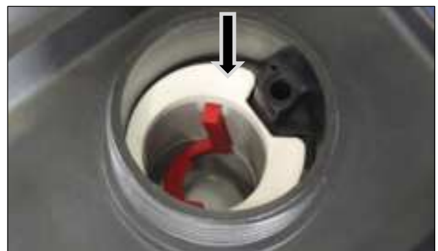
Figure 36 Install the Fuel Strainer
