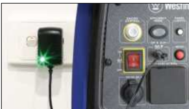
Figure 19 Connect the Battery Charger to Mains Power Supply
