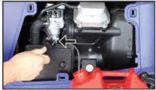
Figure 38 Drain the Carburettor
