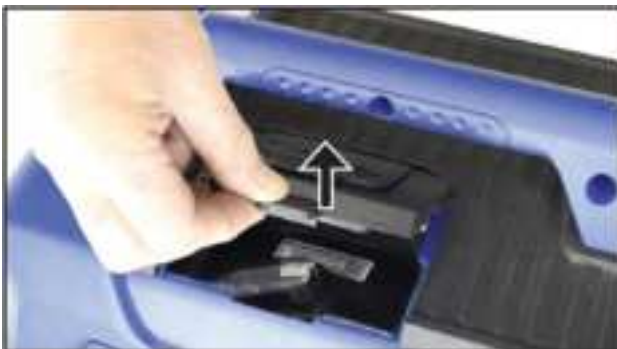
Figure 41 Remove the Spark Plug Access Cover
