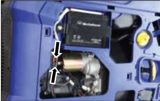
Figure 6 Assemble the Battery Wiring Harness Connector
