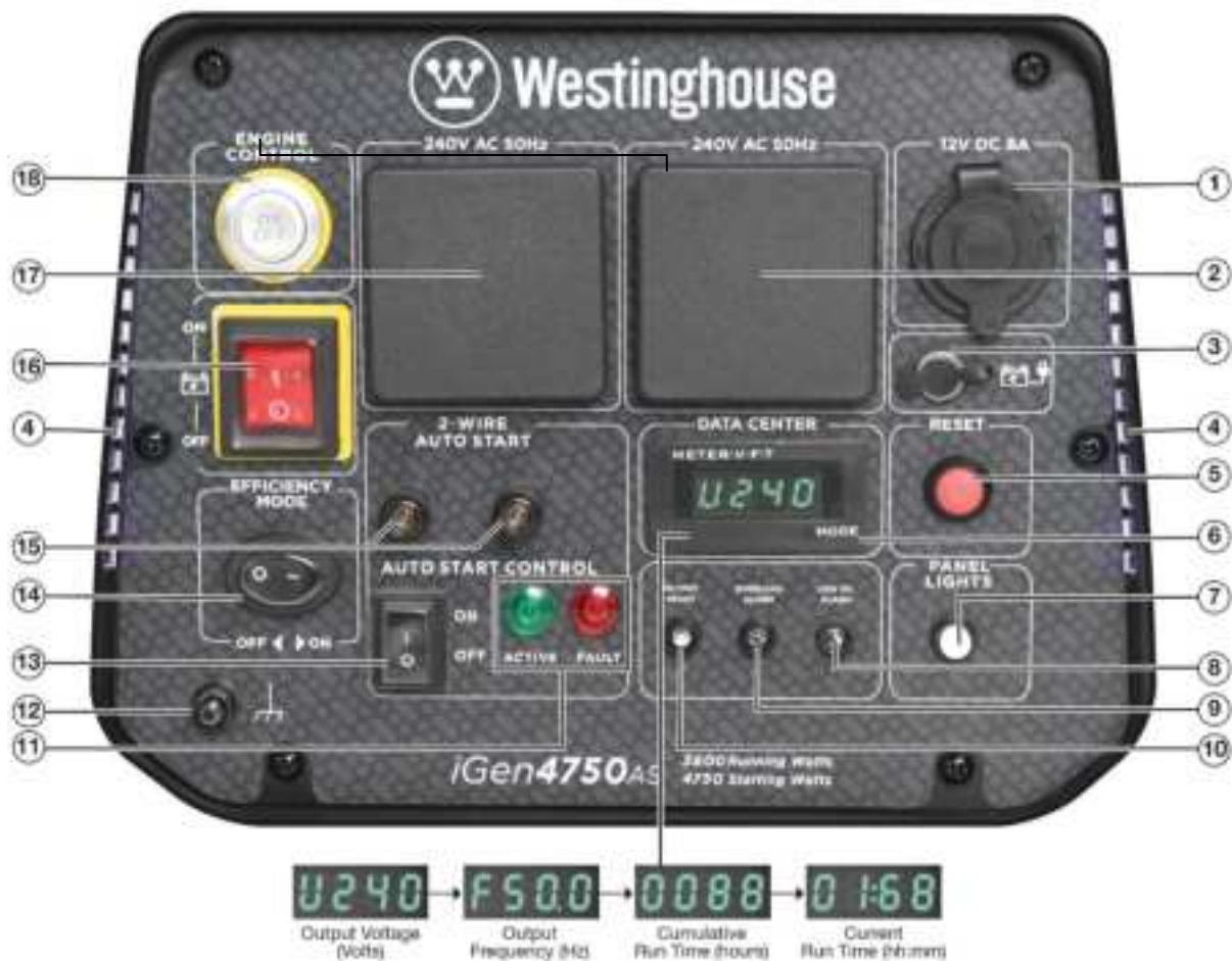
Figure 4 iGen4750AS Control Panel Features
