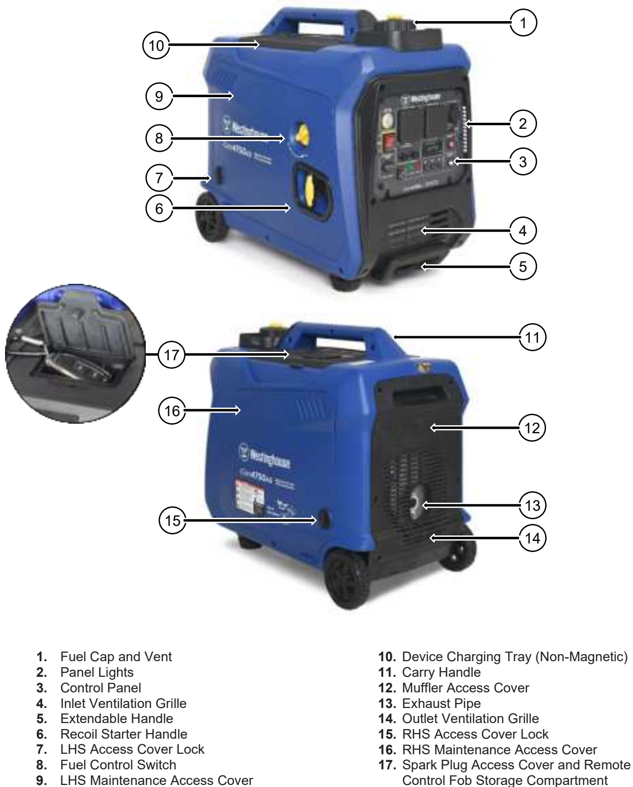
Figure 3 iGen4750AS Main Generator Components
