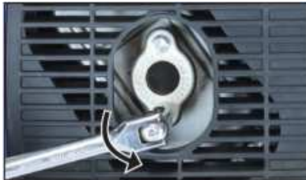
Figure 45 Remove the Spark Arrestor Clamp
