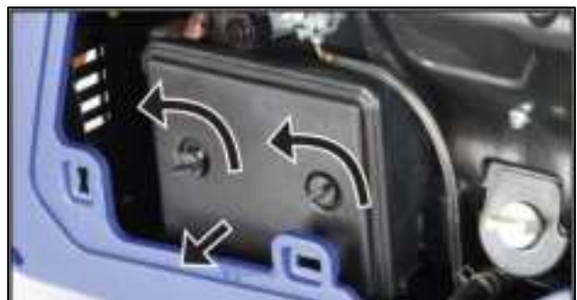
Figure 33 Remove the Air Filter Cover
