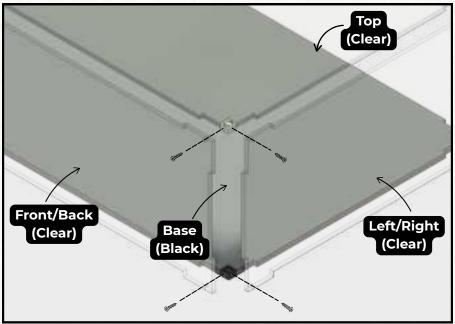
\*\* All side panels have a top and bottom orientation — the deeper cutouts go at the bottom.
