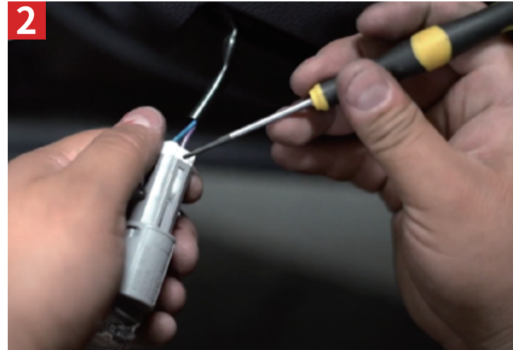
Open the shell of the holder
