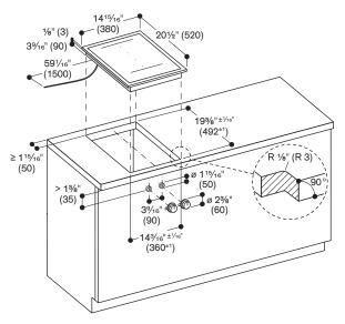
Minimum countertop thickness %'' (20 mm) for surface mounted installation. See separate planning notes on page 104.
