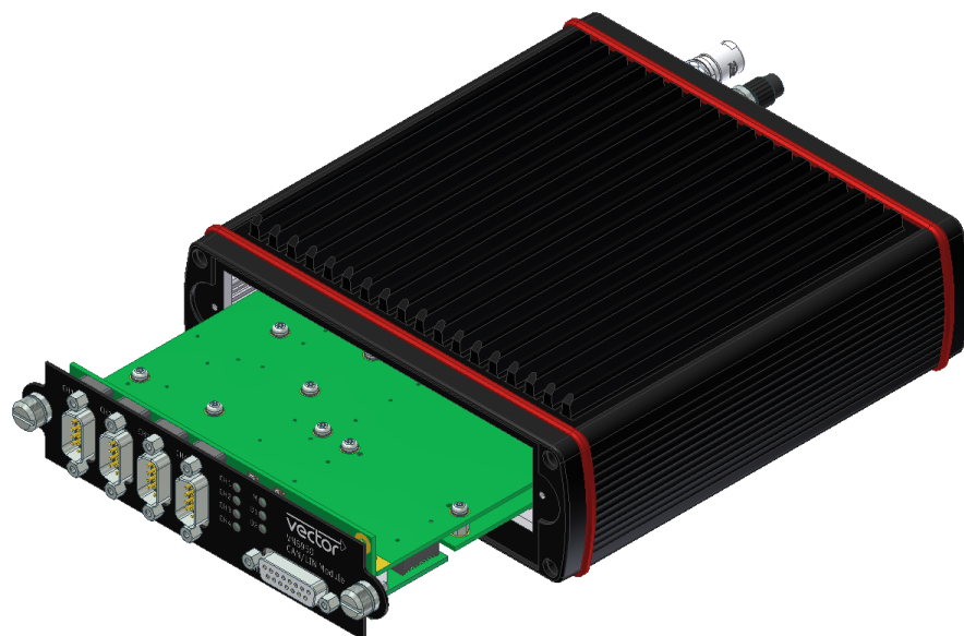
Figure 3: VN8910A with inserted VN8950 CAN/LIN Module
