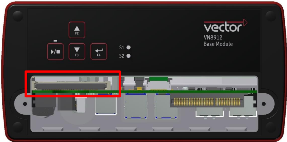
Figure 11: CFAST card slot in VN8912 The VN8912 operating system is stored on a CFAST card and must not be removed during operation.
