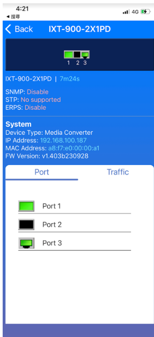
Figure 4-2-50: The screenshot of IXT-900-2X1PD being monitored on a mobile phone
