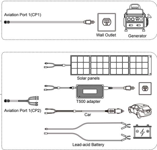
Charging Method 5: Supports charging the AC300+B300 with CP1 and CP2 at same time. You can use any charging methods listed previously, simultaneous, to maximize charging power input. They are listed here again for your convenience. Select one method for CP1 and one method for CP2 for simultaneous charging.
